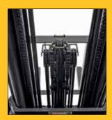
**Forward Visibility**Narrow mast channels and open overhead guard design for excellent visibility.
